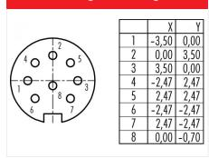
Contact arrangement (Plug-in side)
